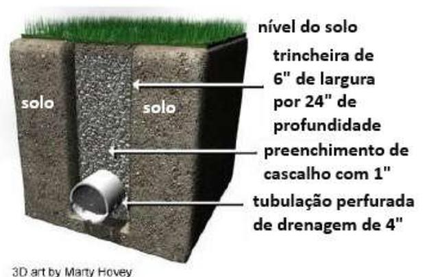
Figura 10: Filtro francês. Fonte: Marty Hovey, in SuDS Wales, c2024h, p. 1. Disponível em: <<https://www.sudswales.com/types/permeable-conveyance-systems/filter-or-french-drains/>>. Acesso em: 22 jan. 2024.
